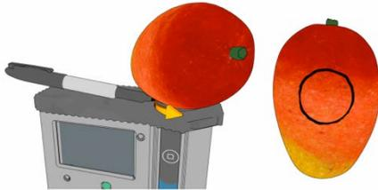
2. On the F-750 with Specimen 1 highlighted on the list, press the right arrow to collect the training spectra. The instrument will indicate “Processing”. **Do not press the scan button to gather training set spectra.**
