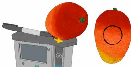
6. On the F-750 with Specimen 1 highlighted on the list, press the right arrow to collect the training spectra. The instrument will indicate "Processing". **Do not press the scan button to gather training set spectra.**
